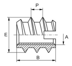
Female thread A = M2,5Length B = 6Male thread E = 5.0Min hole depth = 8Recommended bore diameter (plastic/hard wood) = 3.6 to 3.8Recommended bore diameter, soft wood (largest) = 4.0Thread pitch P = 2.0
